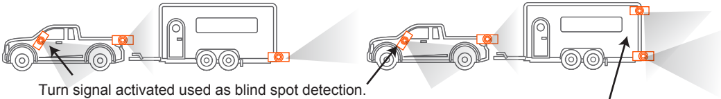
Having two cameras at the back, one camera can be optimised for parking (top down view) whilst the other can look backwards and be used as a rear-view mirror substitute.
