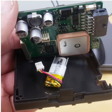
3 Figure 3 Battery connection
